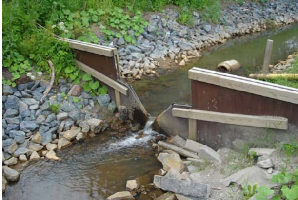
Image 1. Discharge measurement weir upstream from investigated reach during low flow in July 2009.
